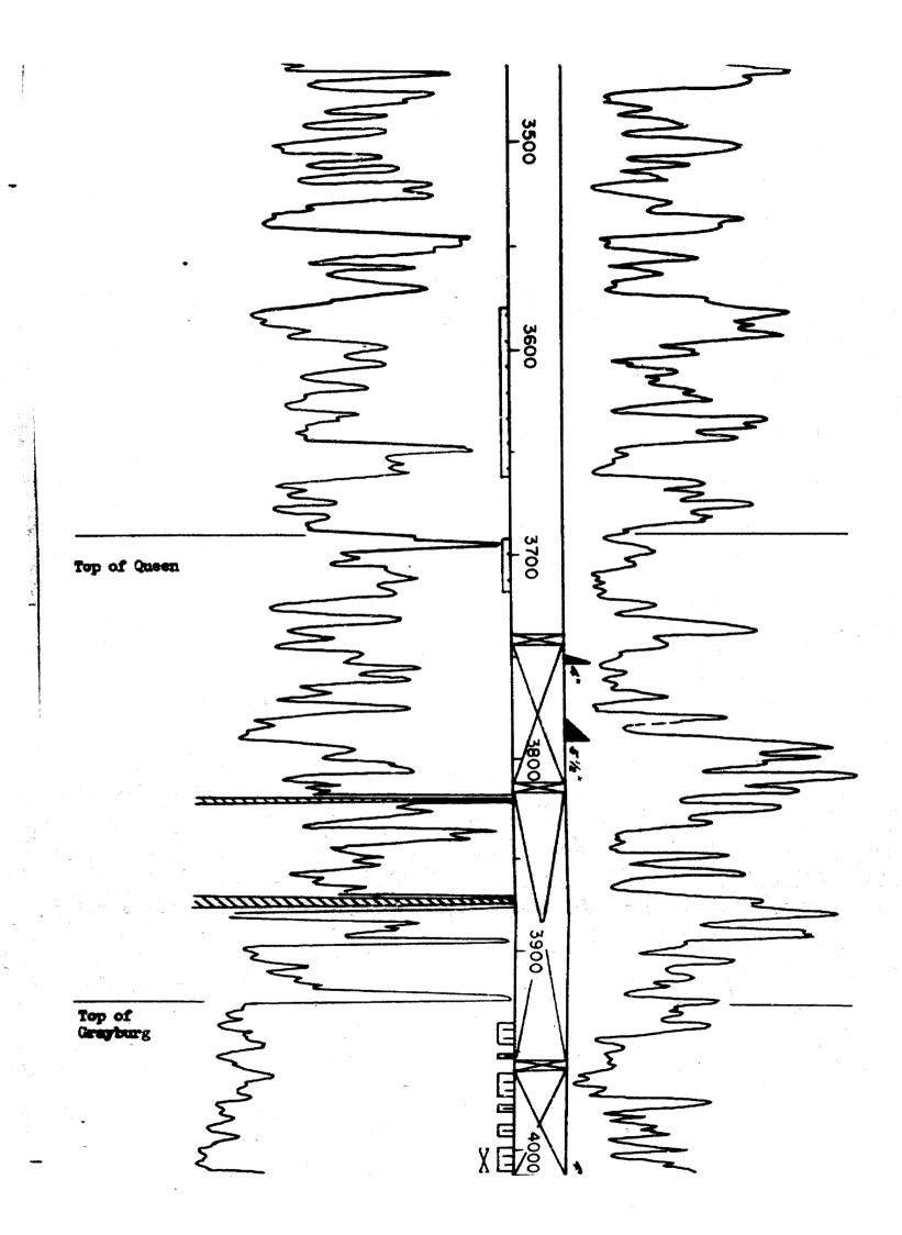
10 3/4" esg @ 100" w/75 mx 7 5/8" esg @ 1775" w/400 mx 5 1/2" esg @ 3797" w/400 mx
