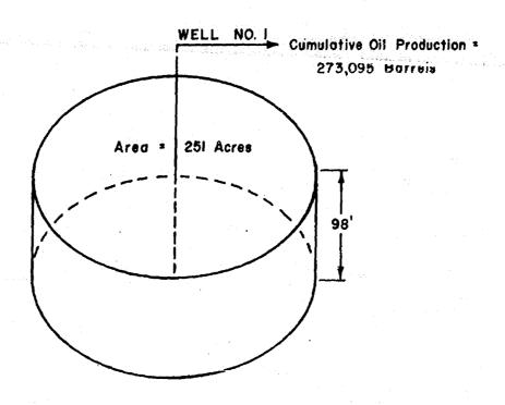
Pressure Decline =  $\frac{N_D}{c_e N} \times \frac{B_O}{B_{O1}}$ Pressure Decline =  $\frac{273,095}{(23.2 \times 10^{-6})(5.04 \times 10^{6})} \times \frac{1.241}{1.185}$ Pressure Decline =  $\frac{338,911}{139}$ Pressure Decline = 2438 psi
