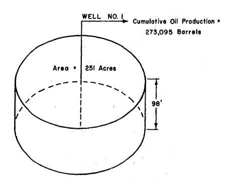
Pressure Decline =  $\frac{N_D}{c_e N} \times \frac{B_O}{B_{oi}}$ Pressure Decline =  $\frac{273,095}{(23.2 \times 10^{-6})(5.04 \times 10^{6})} \times \frac{1.241}{1.185}$ Pressure Decline =  $\frac{338,911}{139}$ Pressure Decline = 2438 psi
