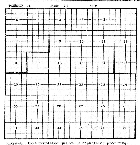
Robert N. Enfield, Bunnel Fed. Well No. 1 in unit J of Section 18-21-23. Completed in Upper Pennsylvanian September 27, 1965, through perforations 7126 to 7133.
