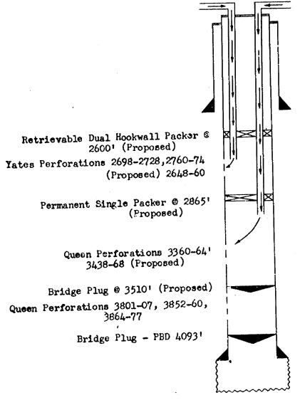
8-5/8" Surface Casing Set At 898". Cemented With 50 Sacks.
