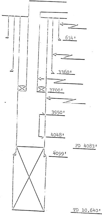
13 3/8" OD casing set at 634' and cemented to surface w/650 sacks.
