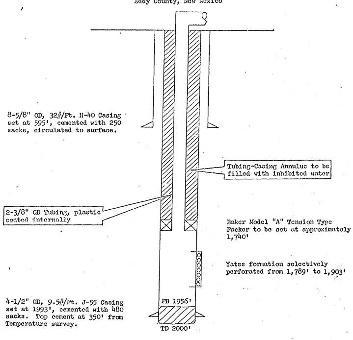
Diagrammatic Skatch Proposed Injection Well
