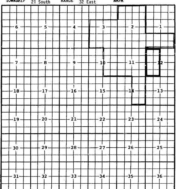
PURPOSE: One completed gas well capable of producing. Belco Petroleum Corporation Federal HM 12 Well #1 in Unit L of Section 12, T21S, R32E. Completed in the Morrow formation on April 14, 1977. Top of perforations 13,958'. Pool boundary outlined in red.
