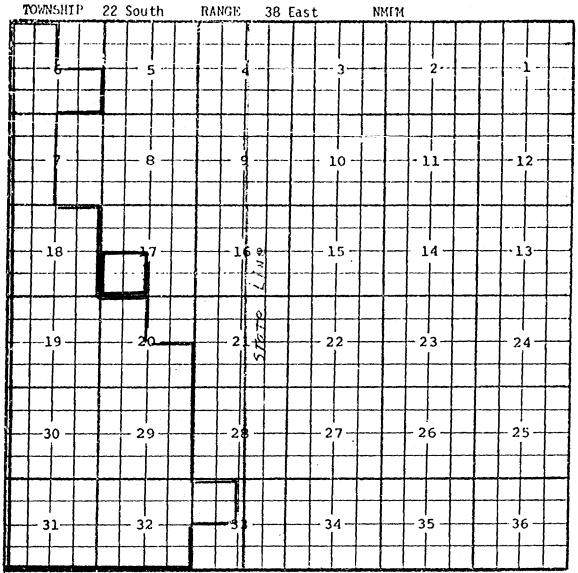
Texaco Inc. Dollie Ballinger Well #1 in Unit M of Section 17, T22S, R38E. Completed June 9, 1977, in the Blinebry formation. Top of perforations 5718'.
