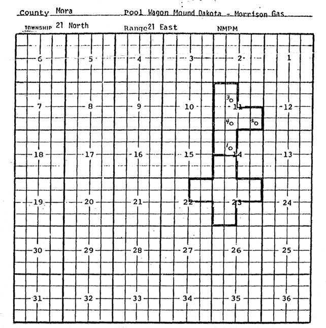
Purpose: Four completed gas wells capable of producing. W. E. Bakke Darwin Daniels Well No. 2 in Section 11, Township 21 North, Range 21 East, completed February 13, 1977, in the Dakota formation. Top of open hole is at 455'.
