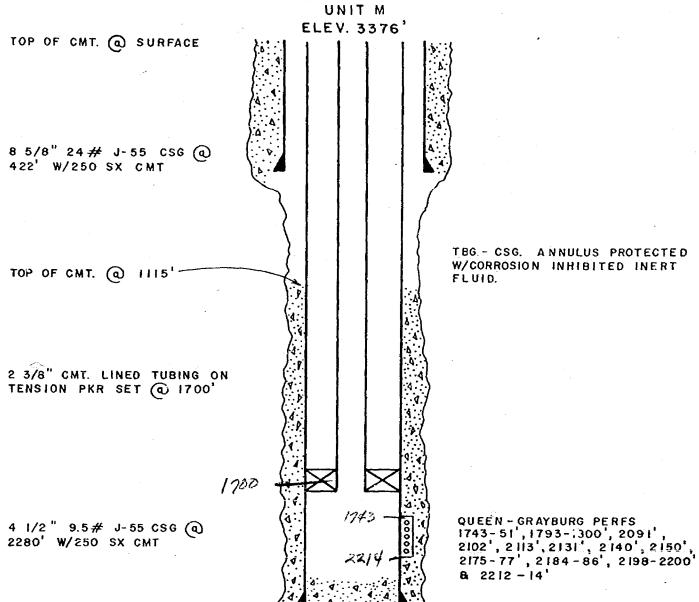
PROPOSED WATER INJECTION WELL (SHOWN IN INJECTION CONFIGURATION)
