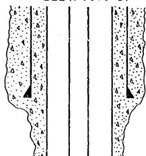
TBG.-CSG. ANNULUS PROTECTED W/CORROSION INHIBITED INERT FLUID
