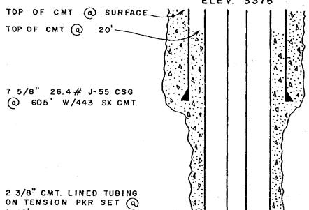
TBG. - CSG. ANNULUS PROTECTED W/CORROSION INHIBITED INERT FLUID
