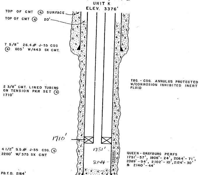
PROPOSED WATER INJECTION WELL (SHOWN IN INJECTION CONFIGURATION)
