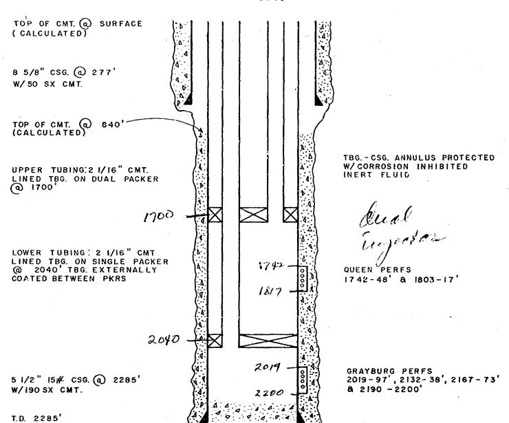
PROPOSED WATER INJECTION WELL (SHOWN IN INJECTION CONFIGURATION)
