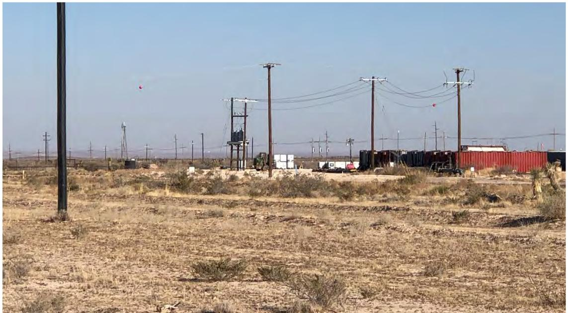
*View east-southeast from the approximate location of Hayhurst Section 2 geotechnical boring B2. This is one of three borings that encountered groundwater about 24 feet below surface. The existing recycling facility is on the right of the image and will be improved when the Gravitas AST is added.*
