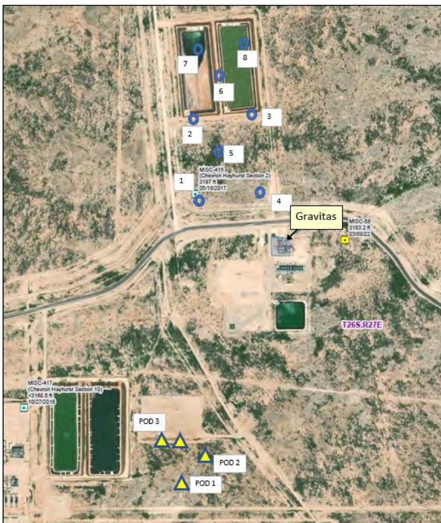
Because groundwater exists in the six borings nearest to the Gravitas AST Containment and the active windmill about 500 feet to the east and groundwater does not exist in the six borings more distant from the windmill and AST, we conclude that shallow groundwater beneath the AST location is localized.
