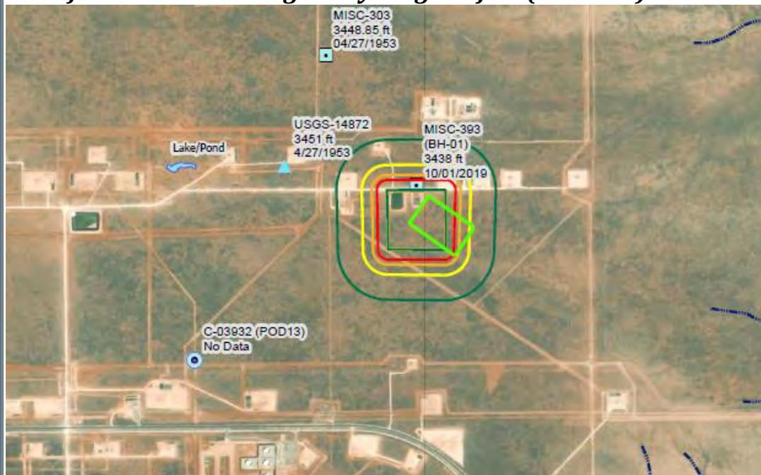
*Location of Revelation recycling project relative to Route 128 and the adjacent Gamma Ridge Containment #1 (1RF-447), which is approved and working as shown in the image. Proposed Revelation Containment (light green rectangle) and AST (between Revelation and Gamma Ridge Containment) lie within large green polygon.*
