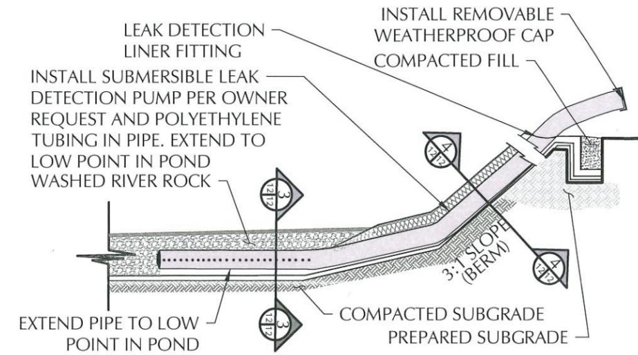
LEAK DETECTION/SAMPLING SYSTEM DETAIL 6
