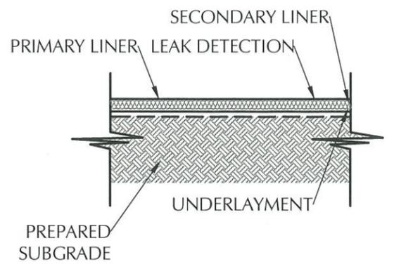
**LINER SYSTEM FLOOR DETAIL** (8) NOT TO SCALE
