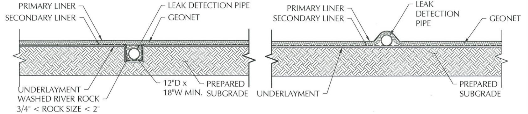
SUMP LEAK DETECTION PIPE DETAIL 3
