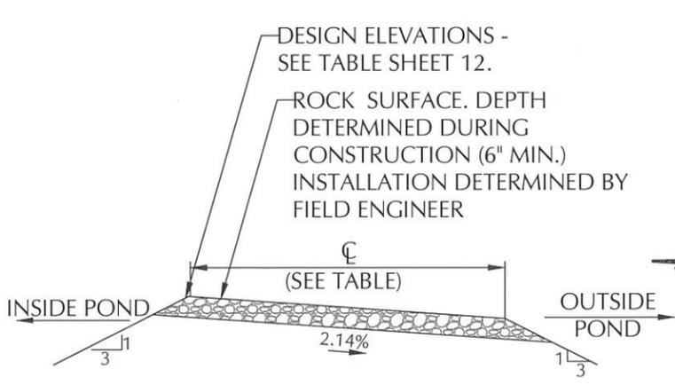
**TYPICAL BERM CREST DETAIL** (10) NOT TO SCALE
