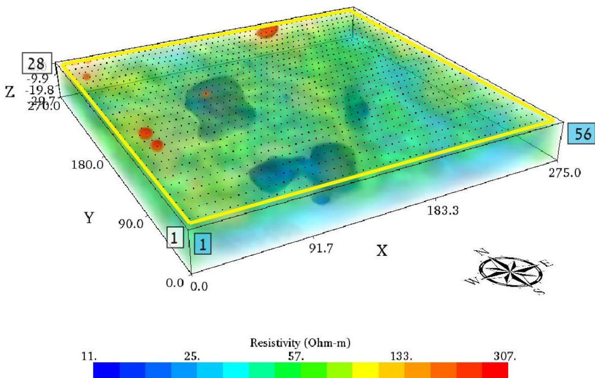
Figure 5: WBRC lines 1 through 28 electrical resistivity oblique 3D volume view showing highest and lowest resistivities. Reds and oranges: higher resistivity. Blues: lower resistivity. Black dots are electrode locations. Red polygons highlight high-resistivity anomalies. Yellow polygon is the proposed pad boundary. Please see APPENDIX 8.3 for more details.
