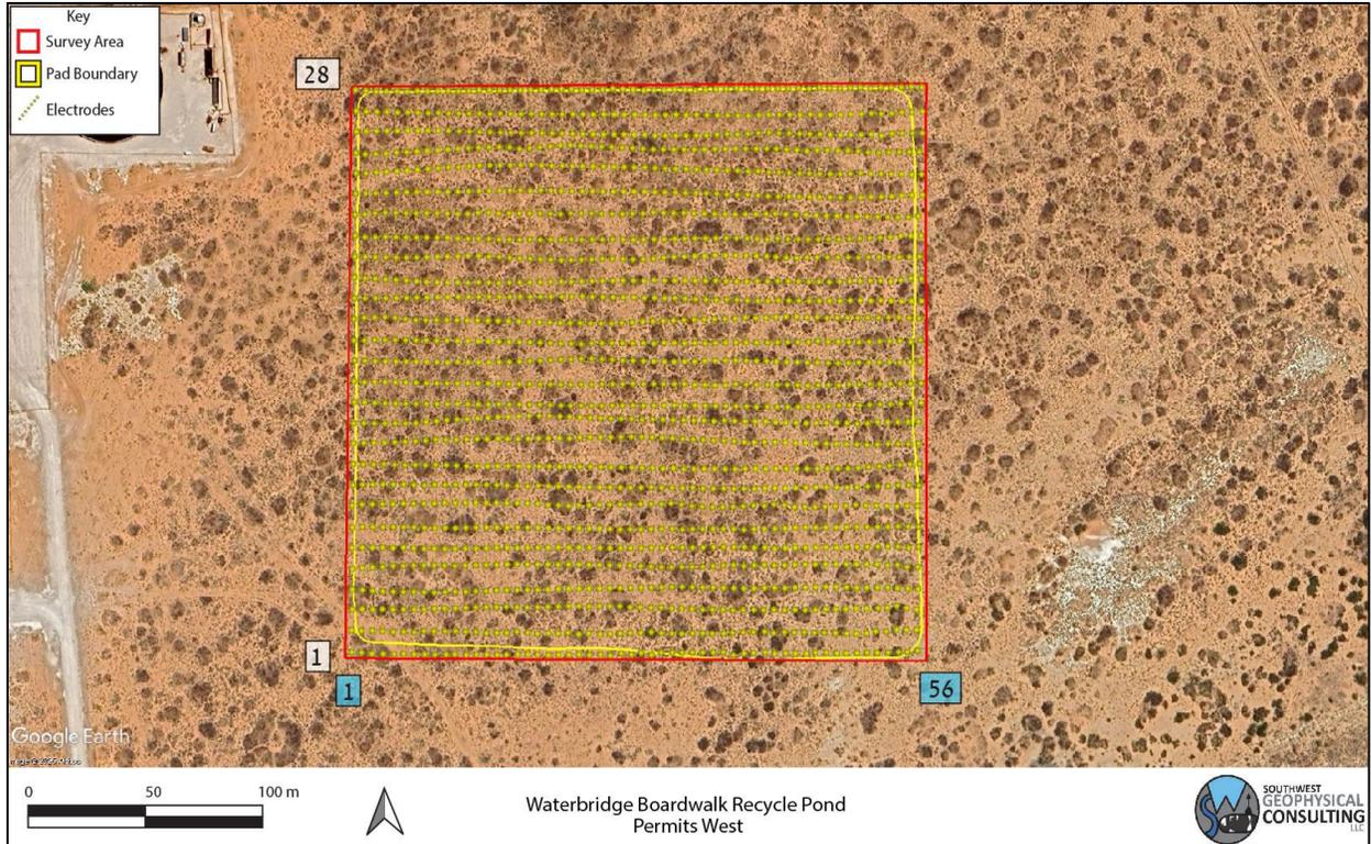
Figure 4: Survey overview. Twenty-eight survey lines (numbered from south to north, in a white background) were conducted at 10-meter spacing, with 56 electrodes at 5-meter electrode spacing (yellow dots, numbered from west to east in a blue background). Background image credit: Google Earth. Image date: July 13, 2024. Image datum: WGS-84.
