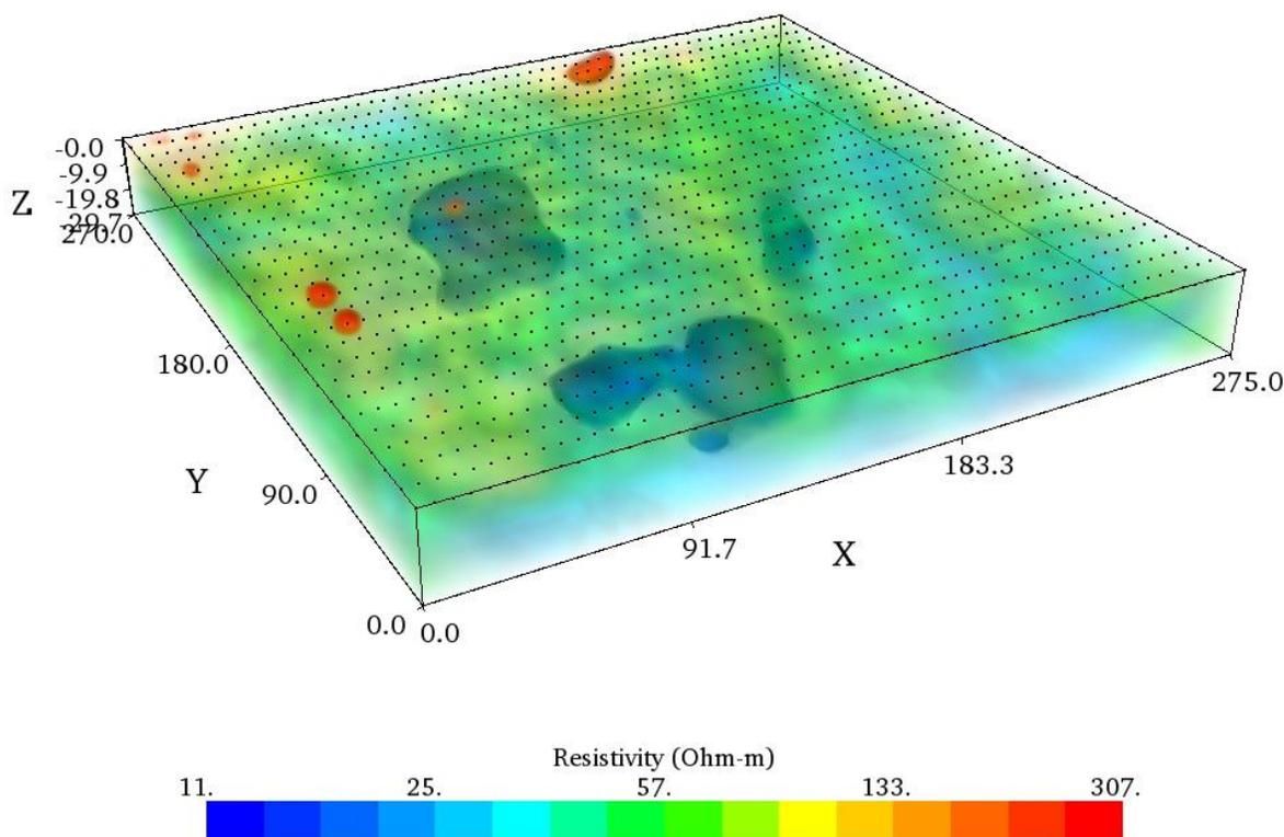
Figure 8: 3D inverted resistivity volume of lines WBRC01 to WBRC28. Small black dots on surface are electrode locations. All axes are labeled in meters.
