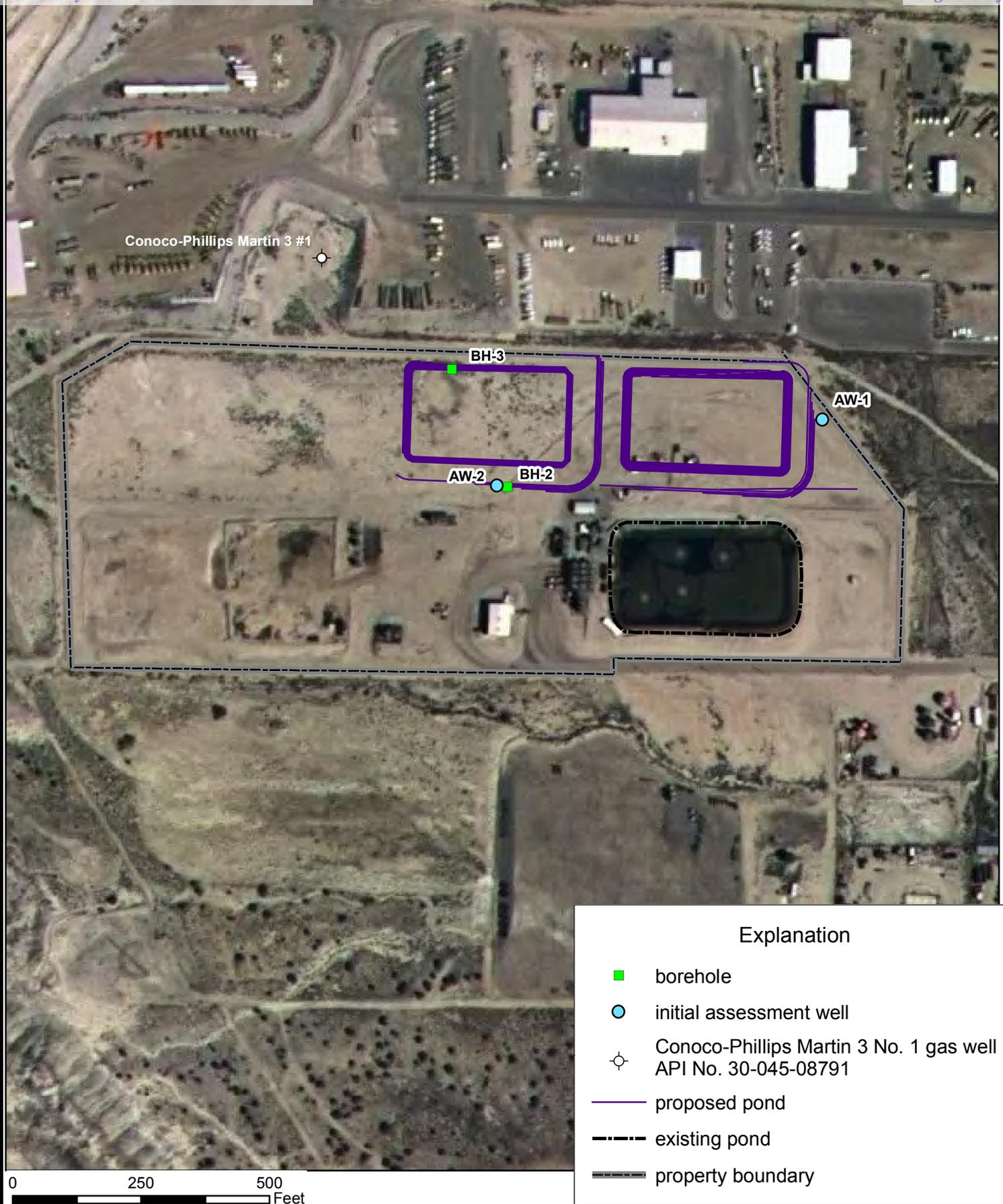
Figure 2. Aerial photograph showing the locations of the existing pond, the drilled boreholes, initial assessment wells proposed evaporation ponds, and well site of the Conoco-Phillips Martin 3 No. 1, Basin Disposal Site, Bloomfield, New Mexico.
