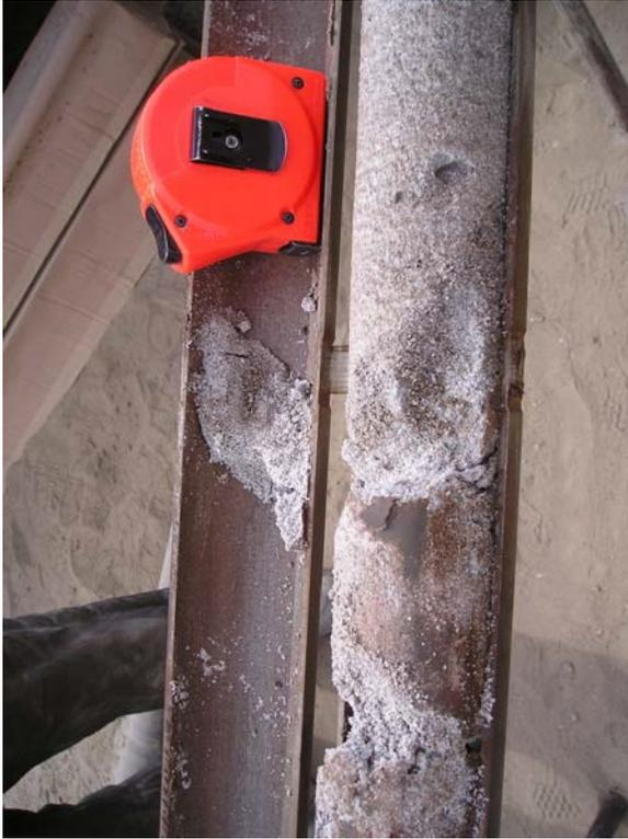
Slightly moist, less consolidated sandstone horizon within the Nacimiento Formation adhering to the core barrel in borehole No. 2 (BH-2).
