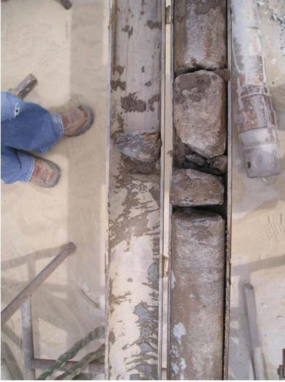
Moist, clay-rich zones, 'missing' from the core and smeared on the core and the inside of the core barrel in borehole No. 2 (BH-2).
