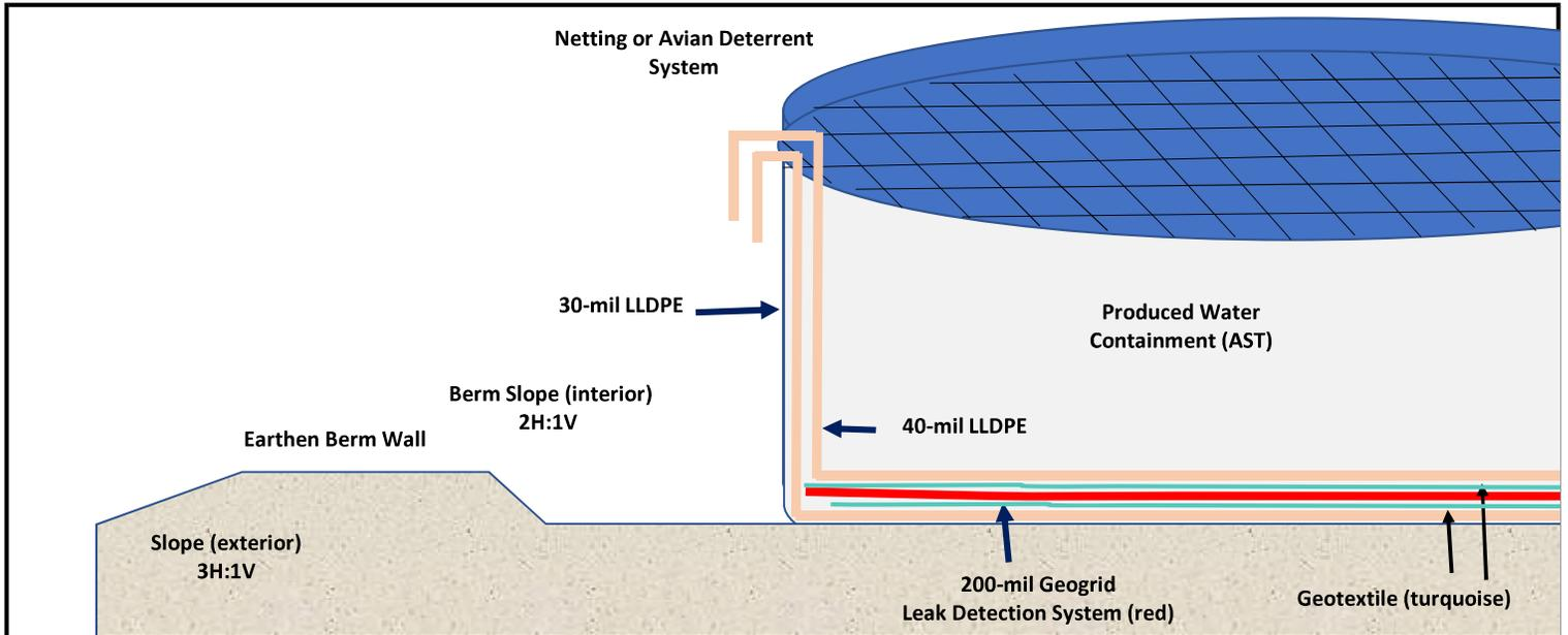
**Description of Leak Detection System**
