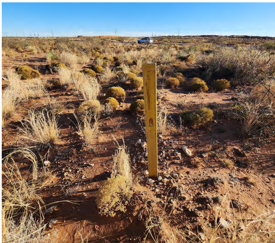
Location 642 looking south along a pipeline on the east side of the AOI. Caliche litters the surface of the buried pipeline demonstrating that caliche underlies the thin aeolian sand.
