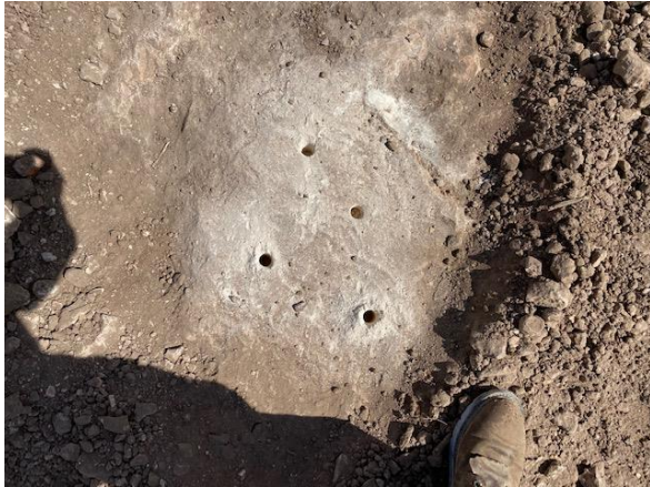
Photograph 13: View of floor sample location taken with hammer drill.
