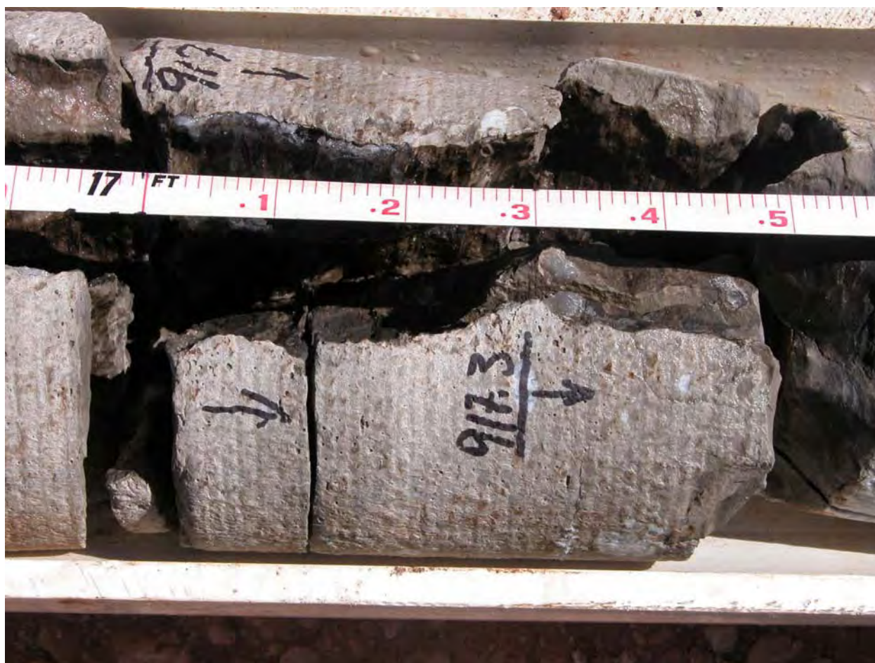
Figure 2-6. Halite on Fracture in Culebra Dolomite. The fracture shows black staining under the clear halite that coats much of the surface. Core has a 4-inch diameter.
