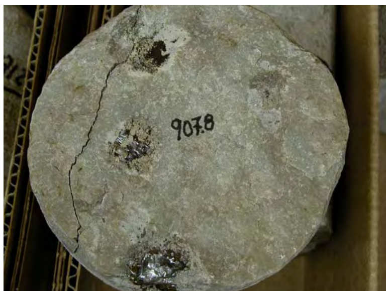
Figure 2-7. Halite in Culebra at 907.8 ft. Halite (dark, clear
