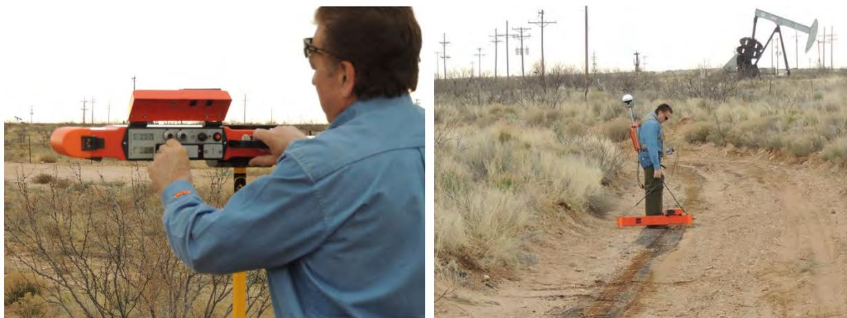
From ECC's review of the conductivity results, it appears that background levels for the WDQSU Sat 3 site range from 3 to 40 mmhos/m. The maximum 0.5-m and 1-m conductivity measurements at the site were 541.95 and 385.70 mmhos/m, respectively.
