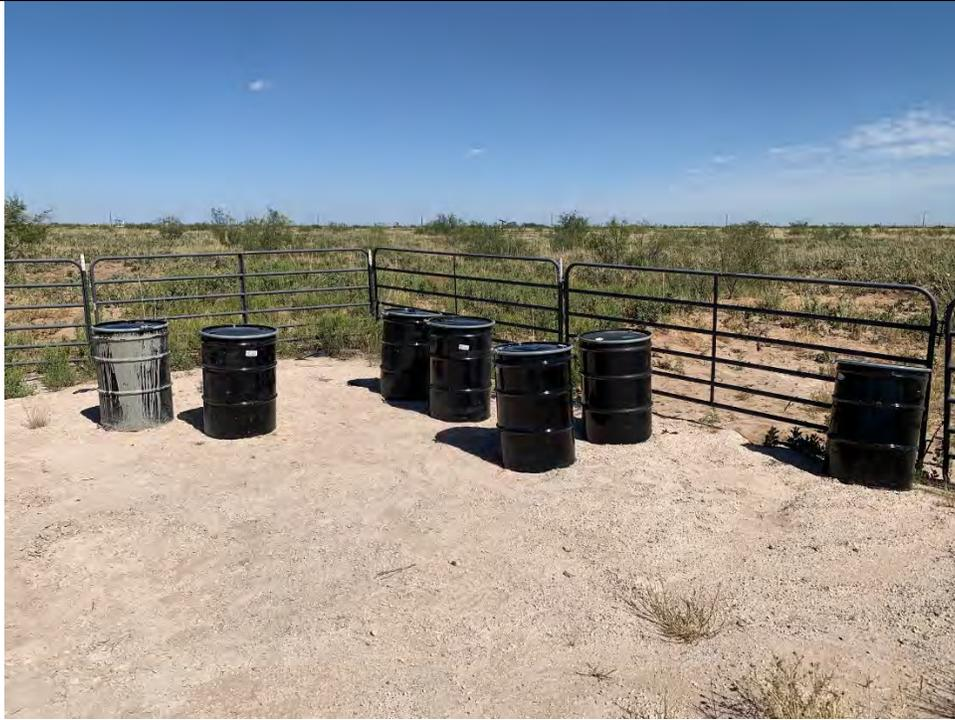
Photo 6: View facing northeast of containerized investigation derived soil, purge water, and trash waste inside seven (7) 55-gallon steel drums. Drums are located within fenced area surrounding release point.
