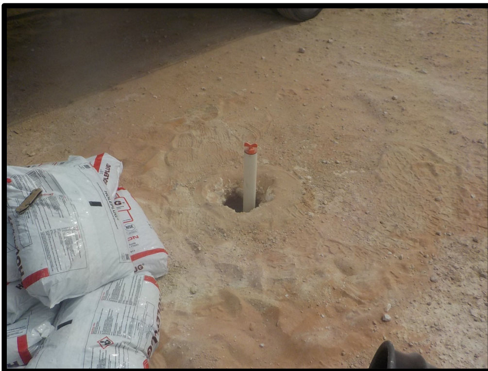
PHOTOGRAPH NO. 3 – A view of the soil boring fitted with PVC casing prior to gauging and plugging and abandonment.
