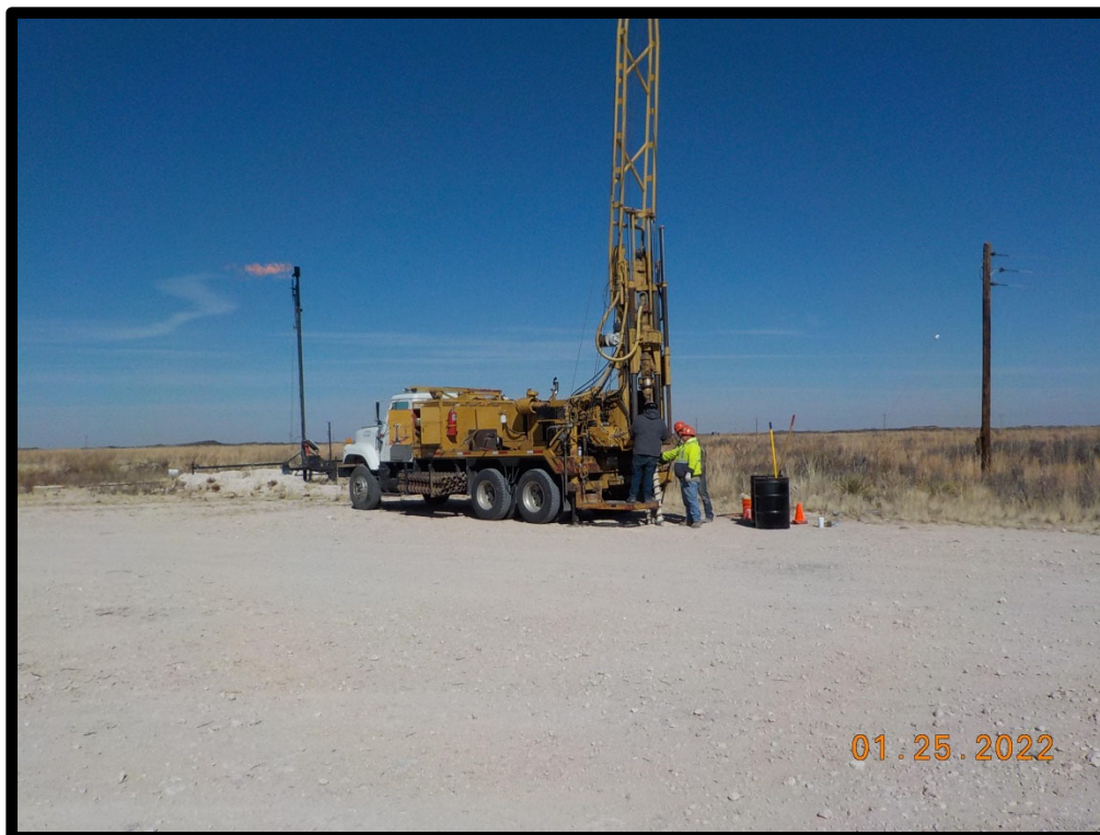
PHOTOGRAPH NO. 1 – A general view of the hollow stem auger soil boring activities on January 25, 2022. The view is towards the northeast.
