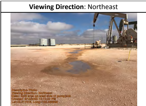
Spill area on west side of pumpjack
