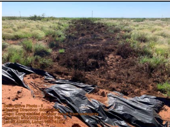
Long stained corridor result from overspray.
