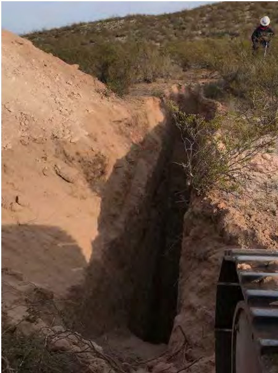
View of pothole PH20 completed at depth 20 feet bgs during background soil sampling activities.
