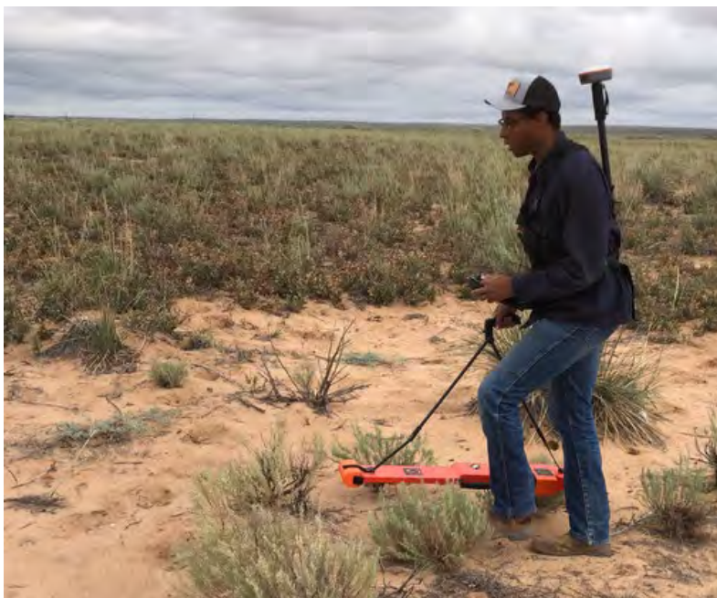
Exhibit 1: Measuring ECa with the EM38 in the horizontal dipole position.
