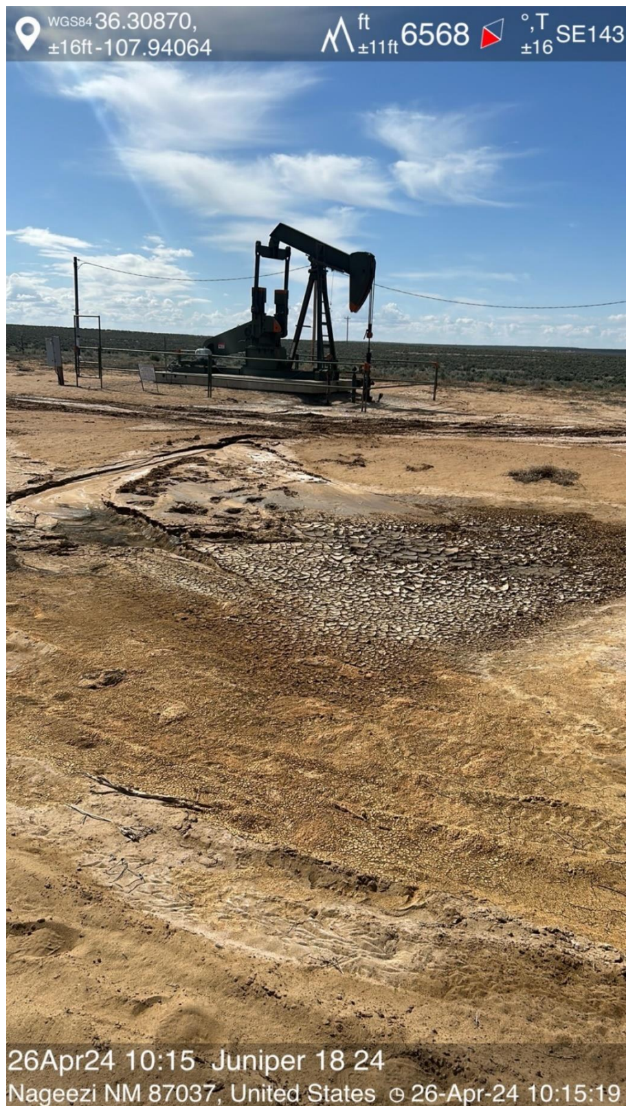
Area north of Juniper 18-24 pumping unit showing discolored and wet soil.
