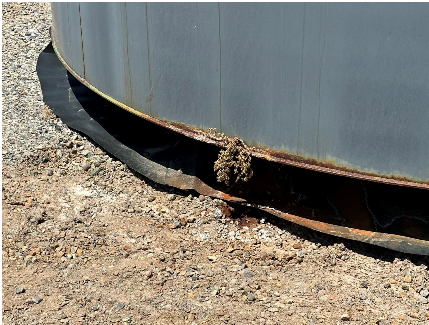
Photo #2 Release point, pinhole corrosion.
