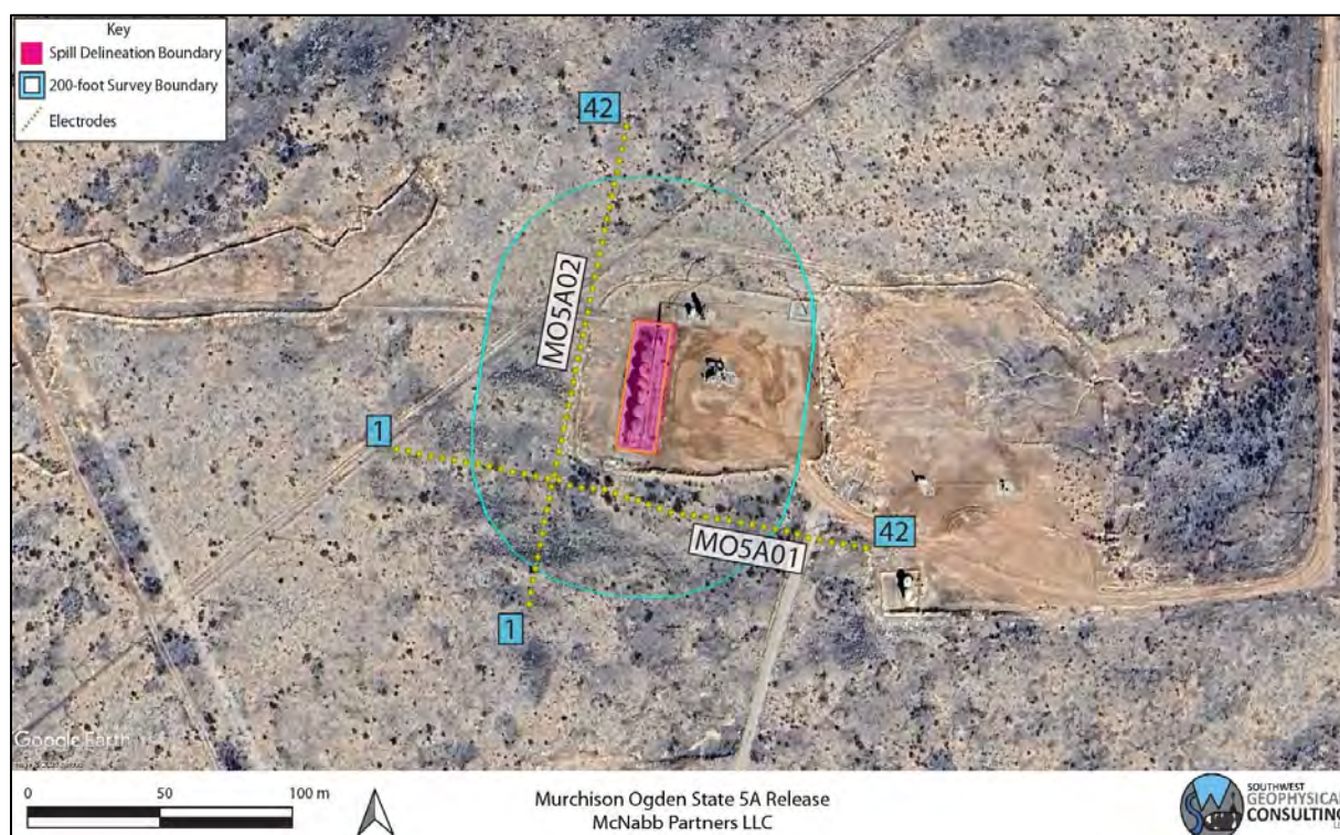
Figure 5: Geophysical survey overview. Two survey lines were conducted with 42 electrodes each at 5-meter spacing (yellow dots denoted with blue numbers). Background image credit: Google Earth. Image date: January 27, 2023. Image datum: WGS-84.
