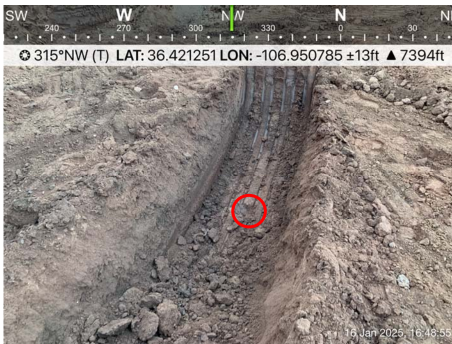
Photo 26: SS21 collected as a discrete sample 12 ft bgs from pothole in southwest corner of excavation.
