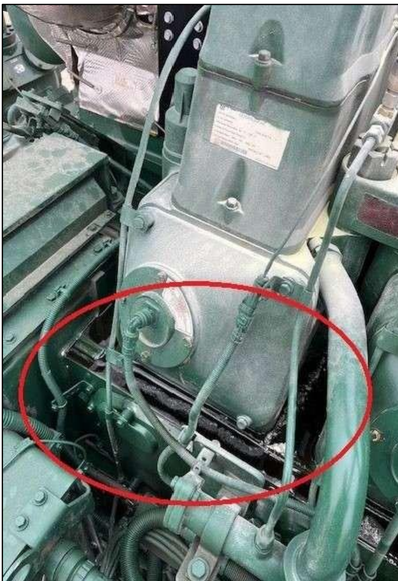
Photo of unit 2519 with the burnt oil stain that was cleaned following the fire event.
