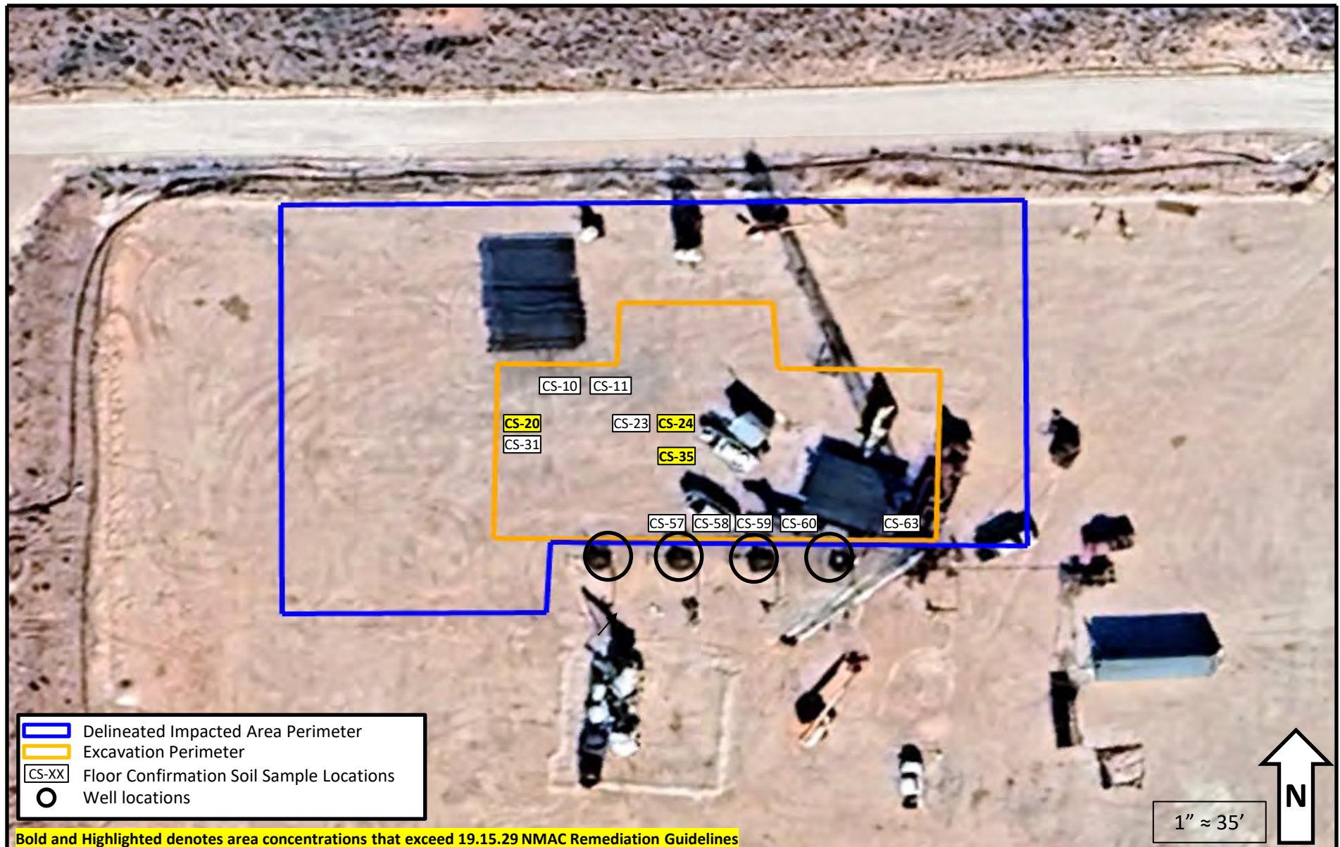
Figure 5 - Confirmation Soil Sample Locations and Site Map (07/09/2024)
