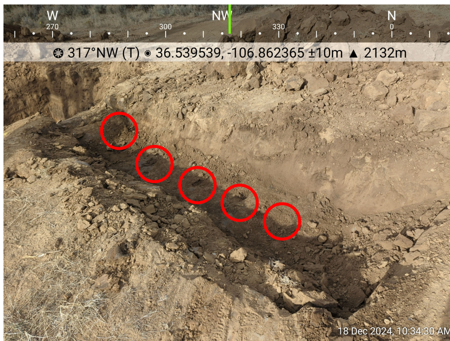
Photo 11: SS08 collected as a 5-point composite sample from new release excavation area.
