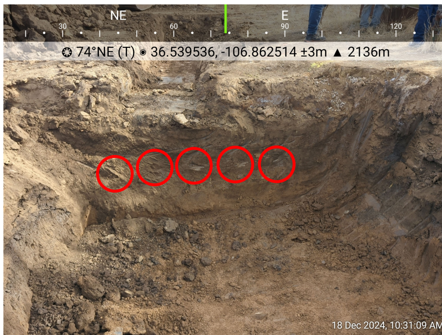
Photo 7: SS04 collected as a 5-point composite sample from east sidewall of wellhead excavation area.
