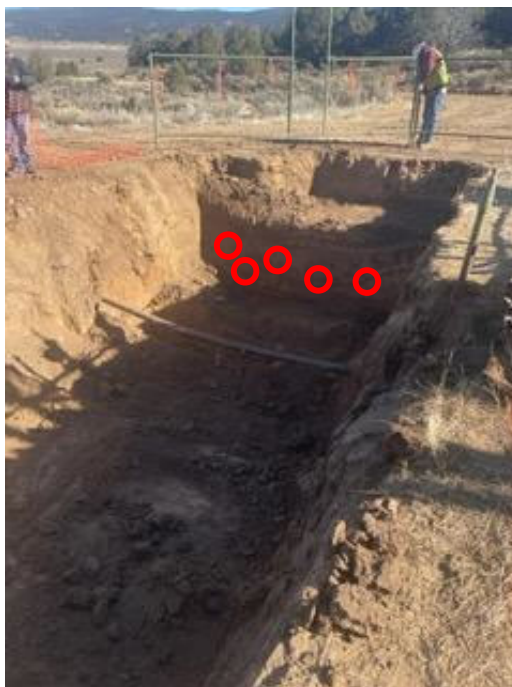
Photo 13: SS09 collected as a 5-point composite from east sidewall of wellhead excavation area 12/23/2024.
