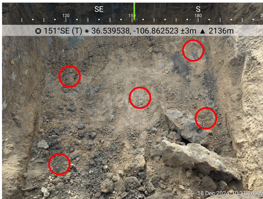
Photo 9: SS06 collected as a 5-point composite sample from the base of wellhead excavation area.
