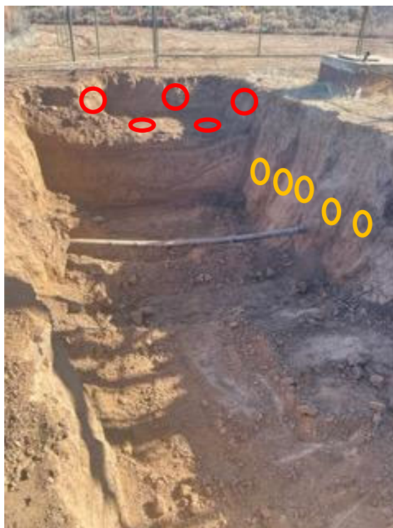
Photo 14: SS10 (red) collected as a 5-point composite from new release excavation area and SS11 (yellow) collected as a 5-point composite from south sidewall of wellhead excavation area, 12/23/2024.
