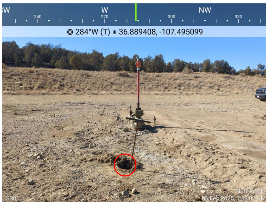
Photo 3: SS01 collected as a vertical delineation grab sample 3.5 feet below ground surface, adjacent to the point of release.
