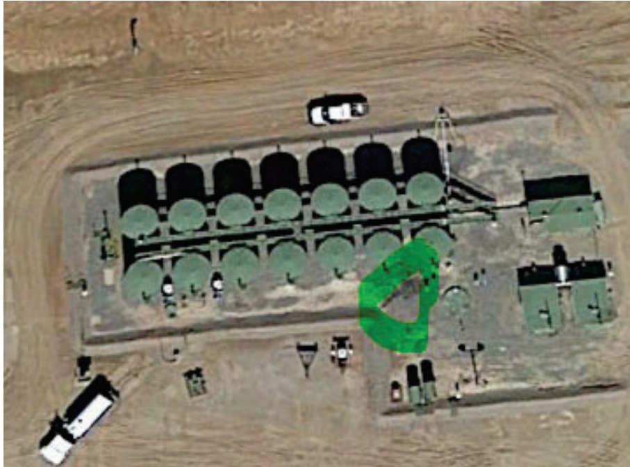
Photo 13: 2016 aerial documenting potential spill in containment, this area must be assessed.
