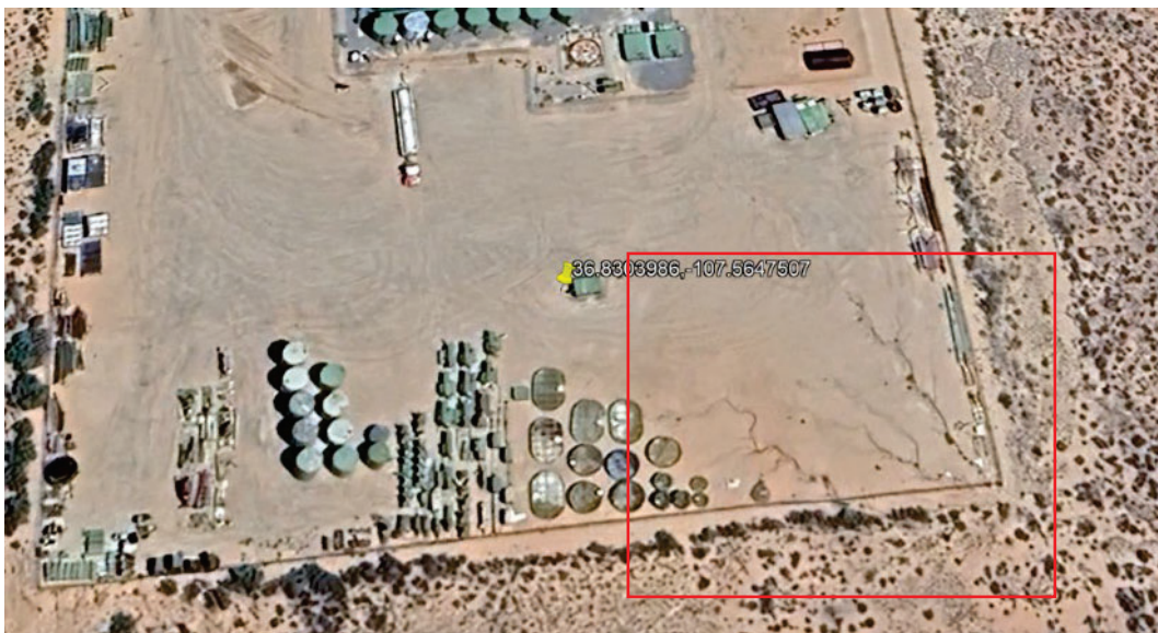
Photo 5: Erosion on southeast corner of facility.
