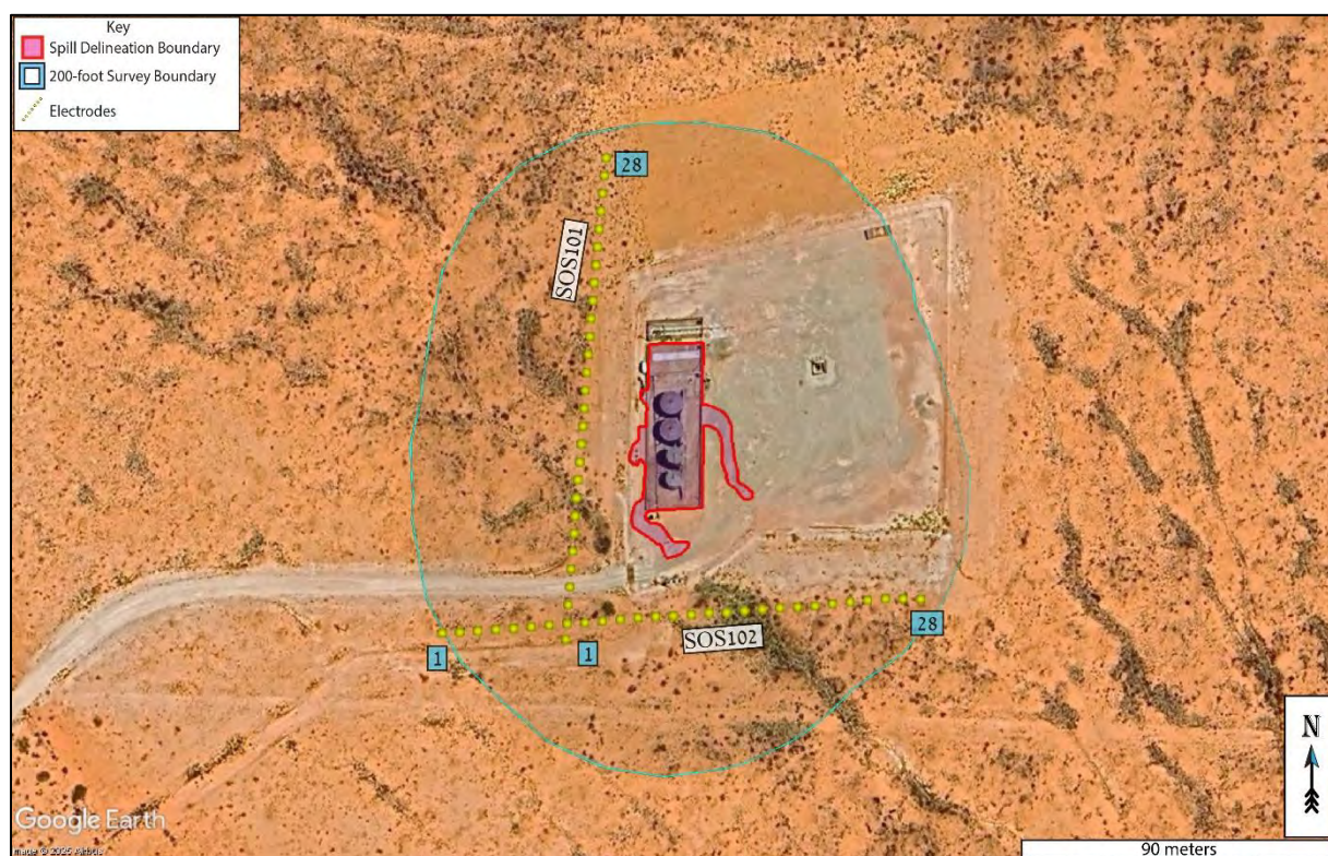
Figure 5: Geophysical survey overview. Two survey lines were conducted with 28 electrodes at 5-meter spacing (yellow dots denoted with blue numbers). Background image credit: Google Earth. Image date: August 13, 2024. Image datum: WGS-84.
