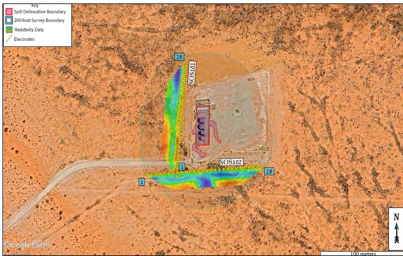
Figure 8: Data overlay. Colored trapezoids are the 2D inverted resistivity line. Background image credit: Google Earth. Image date: August 13, 2024.
