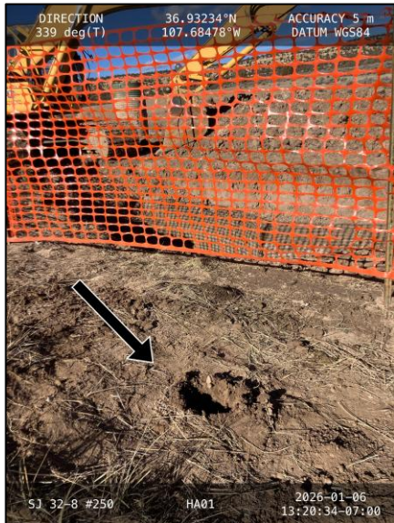
Photograph: 1 Date: 01/06/2026 Description: Hand auger boring, HA01, advanced adjacent to the valve can (source of release). View: North
