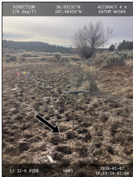
Photograph: 3 Date: 01/07/2026 Description: Hand auger boring, HA03, advanced within the release footprint. View: South
