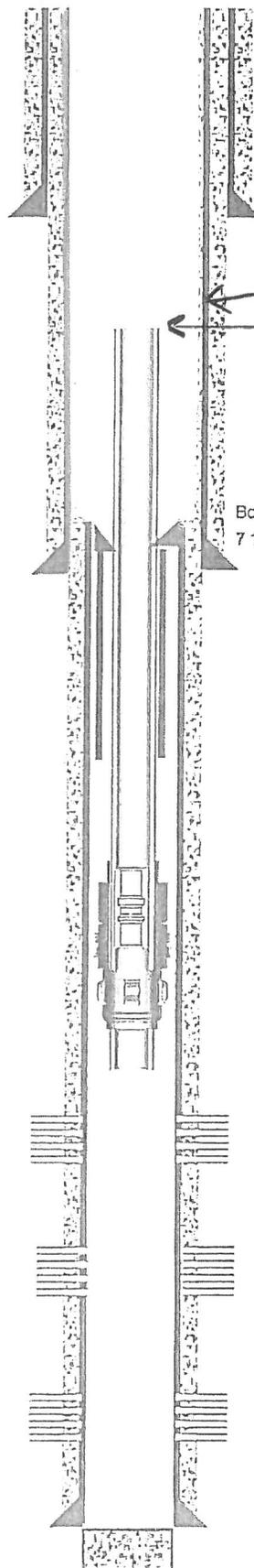
Collapsed 9-5/8 casing @ ~ 1980'
