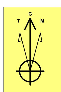
**Azimuths to Grid North** True North: -0.43° Magnetic North: 6.27°
