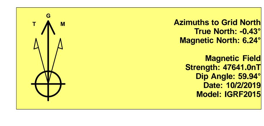
To convert a Magnetic Direction to a Grid Direction, Add 6.24° To convert a Magnetic Direction to a True Direction, Add 6.67° East To convert a True Direction to a Grid Direction, Subtract 0.43°
