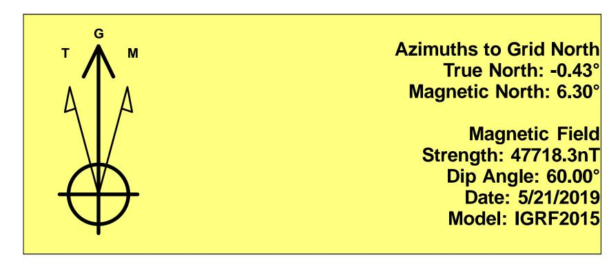
To convert a Magnetic Direction to a Grid Direction, Add 6.30° To convert a Magnetic Direction to a True Direction, Add 6.72° East To convert a True Direction to a Grid Direction, Subtract 0.43°
