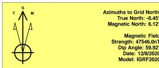
To convert a Magnetic Direction to a Grid Direction, Add 6.12°
