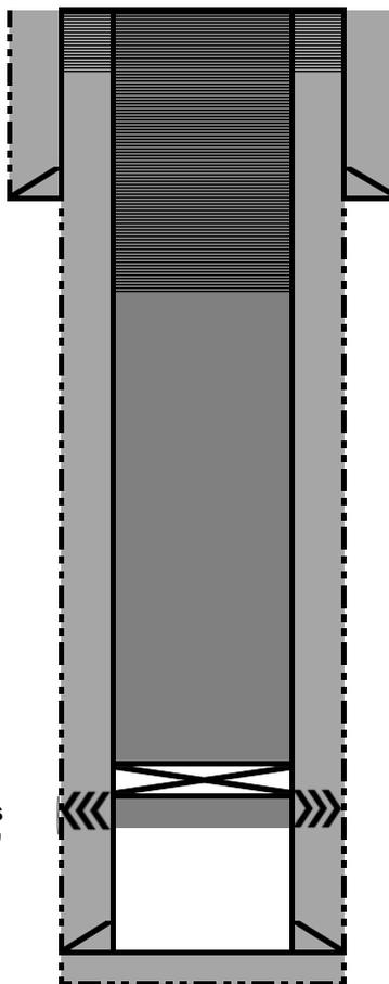
**Plug 3:** Top off plug, Mix and pump 42 sx class G cement into casing and annulus with 1" poly pipe.
