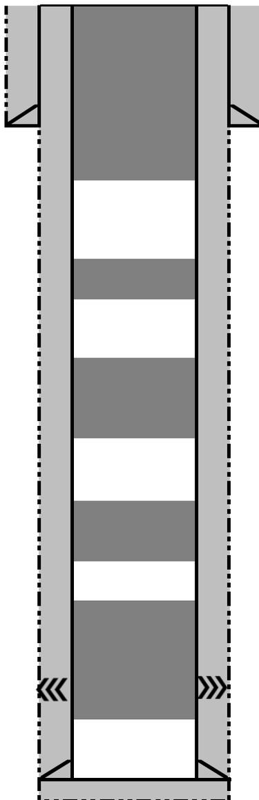
**Plug 5:** Fruitland, Kirtland, Ojo Alamo, surface casing shoe, to surface. Spot 1279' Class G cement plug from 1279' to surface.
