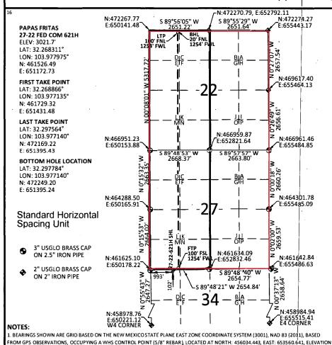
2. DISTANCES DEPICTED HEREON ARE REPORTED AS GROUND DISTANCE IN US SURVEY FEET USING A COMBINED SCALE FACTOR OF 1.000220979
