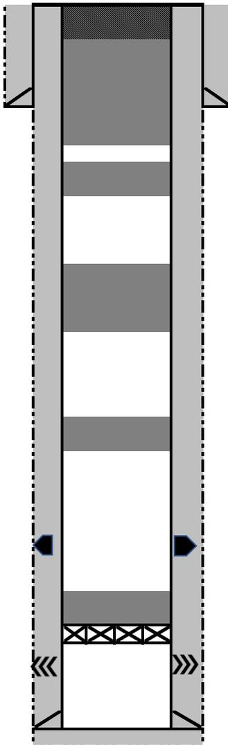
8-17-2020: Top off plug. Mix 18 sx Type II cement to top off.
