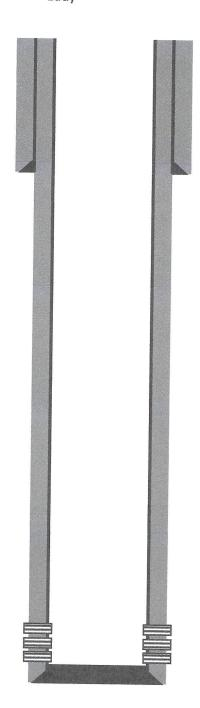
12-1/4" hole @ 1825' 9-5/8" csg @ 1825' w/ 1375sx-TOC-Surf-Circ
