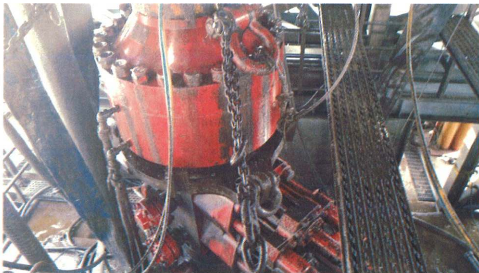
Figure 1: Winch System attached to BOP Stack
