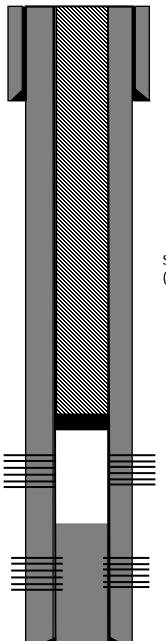
7", 26# Casing Set @ 122'. Cemented w/50 sks Class B. Circulate 2 bbl cement to surface. Hole size 9-1/8"
