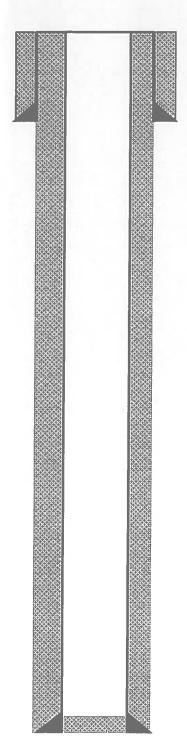
8-5/8", 24# J-55 Casing set @ 120' RKB Cemented w/ 100 sks Class B cement w/ 2% Calcium and ¼#/sk CF Circulated 8 bbl cement to surface
