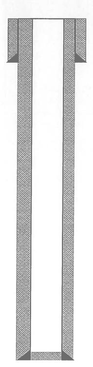
8-5/8", 24# J-55 Casing set @ 120' RKB Cemented w/ 100 sks Class B cement w/ 2% Calcium and ¼#/sk CF Circulated 8 bbl cement to surface
