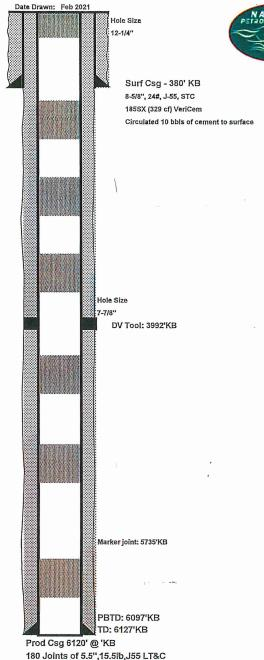
Prod Csg 6120' @ 'KB 180 Joints of 5.5",15.5lb,J55 LT&C CMT: LEAD: 165SX(322cf) Halliburton Lite Prem, TAIL: 205SX(269cf) 50/50 POZ CIRC 50BBL CMT to surface
